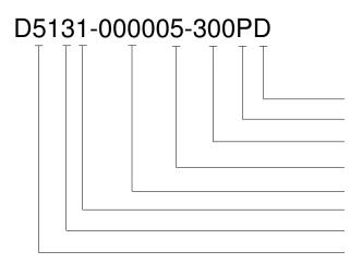
Type (D = Differential) Units (P = psi, B = Bar) Pressure Range (See Pressure Range Table) Pressure Port (See Pressure Port Options Table) Specials (nnnn = Custom Drawing) Connection (See Electrical Connections Table) Output (See Output Options Table) Model
